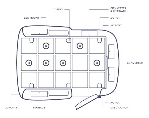
The modular floor of the HC1 is made of 1.5" thick honeycomb fiberglass. Grooves are embedded in the floor to hold the Adaptiv $^{\text{\tiny{M}}}$  cube components in place — just like Lego $^{\text{\tiny{B}}}$ . The surrounding benches are permanent, providing a 42 sq ft walkable space and a total of 72 sq ft of space.
