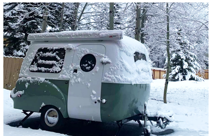
Be sure to drain (and sanitize) your water lines, close all the windows and fan openings, and unplug the battery before storing for winter.
